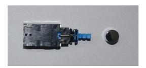
2. Solder SW1 (supplied with the Kit), Chrome cap can be installed prior to soldering
