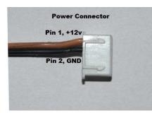
6. Solder the Power cable to Hermes J10 pin1 (+12V), Pin2 (GND), the connector on the other end of the cable plugs into the PA board power connector
