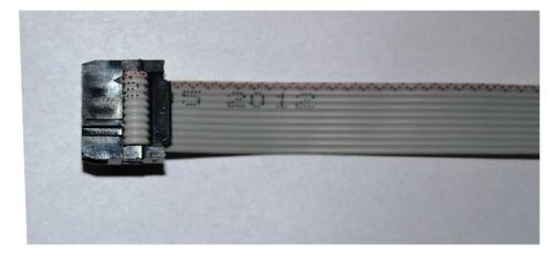
9. Connect the ribbon cable from Hermes J15 to PA connector J7, ensure polarity correction (cable supplied with Kit), ensure that the flat side faces pin 1 on both boards.
